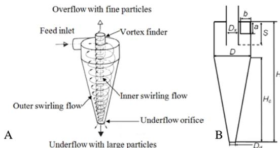
Figure 1. (A) A typical hydrocyclone configuration and flow pattern [14]; (B) Schematic of a hydrocyclone with the characteristic dimensions in the vertical plane [20].
